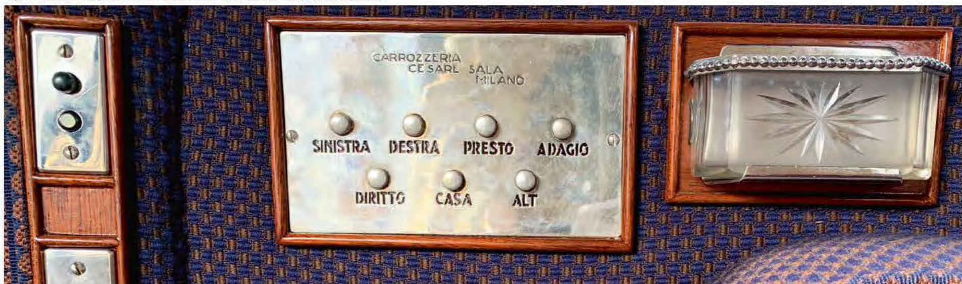
1927 Isotta Fraschini 8A. Chauffeur signal and command panel.
